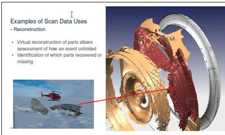
Further, 3D models can be overlaid to reference data such as Catia models or scans of reference parts so that an analysis can be made on how a part had distorted or deformed.
