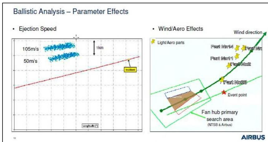
The fan hub primary search area shown above was identified using both Ariane and NTSB ballistic analyses, which were largely consistent.
